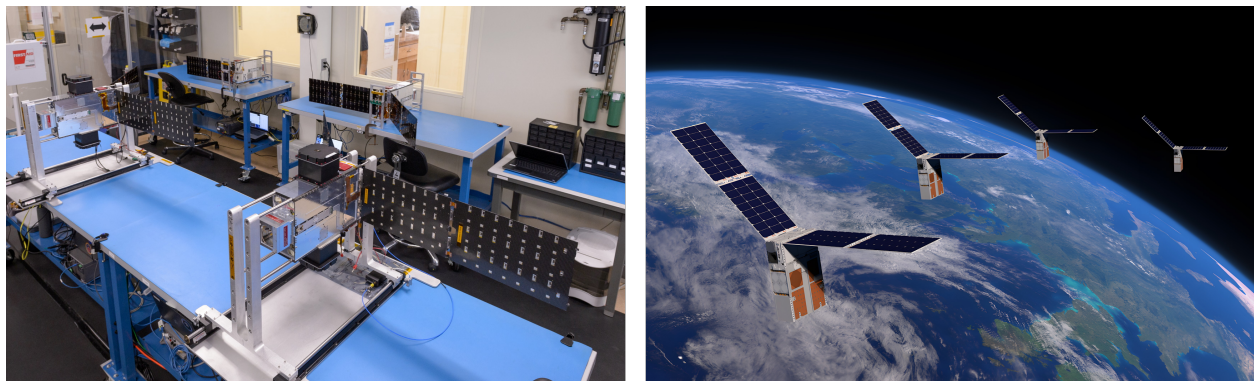
Fig. 5: The four Starling CubeSats during integration (left) (credit: NASA / Dominic Hart) and an artist’s impression of the Starling swarm (right) (credit: NASA / Blue Canyon Technologies).
