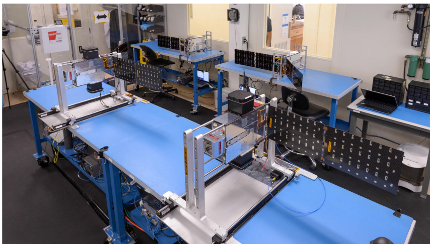
Fig. 10 The four Starling CubeSats during integration. Image courtesy of NASA/Dominic Hart (2022).
